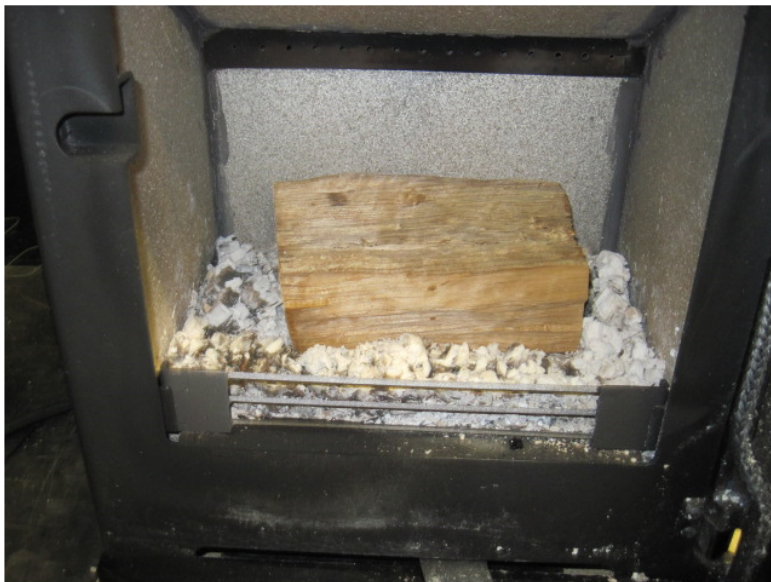
Picture 1 Positioning of the wood during the nominal tests
